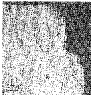
Fig. 8 Details of cross section through the visually observed surface crack etched with Keller's reagent.
